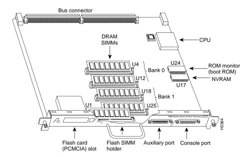
Figure 3 7000 Route Switch Processor (RSP7000)
